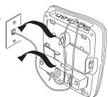
7. On the base, pull the handset retainer out of the slot. Rotate clockwise 180°.
